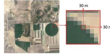
**SPATIAL RESOLUTION:** The observing system must provide **high spatial resolution** (30 and 60 m for VSWIR and TIR)
